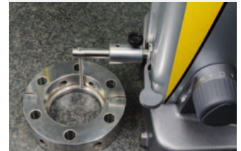
Measurement of the vertical depth of a shoulder
